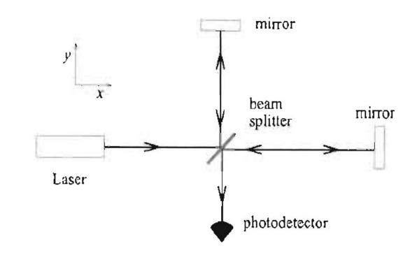
$$E_{\text{out}} = E_1 + E_2 = -iE_0 e^{-i\omega_L t + ik_L(L_x + L_y)} \sin[k_L(L_y - L_x)]$$
